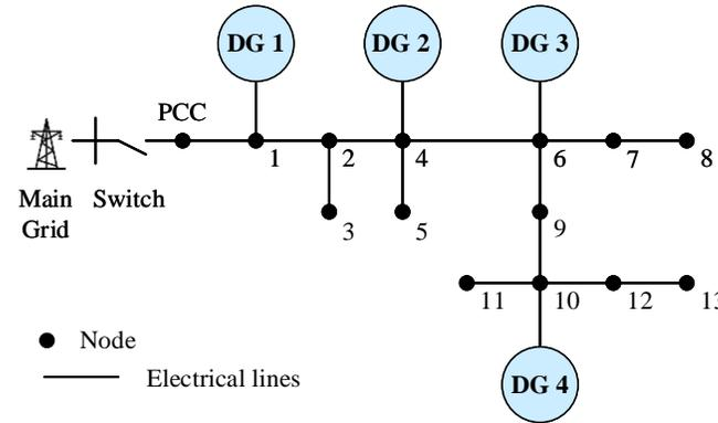
Figure. The topology of the 13-bus microgrid system.
