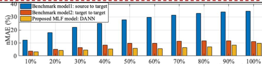
At the lower DER penetration levels, accuracy improvement by TL is not significant since the load is just slightly masked (data distribution is not changed much). With growing DER levels, effectiveness of TF is more and more evident.
