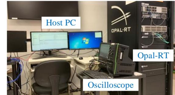
Figure. Real-time experimental test based on Opal-RT.
