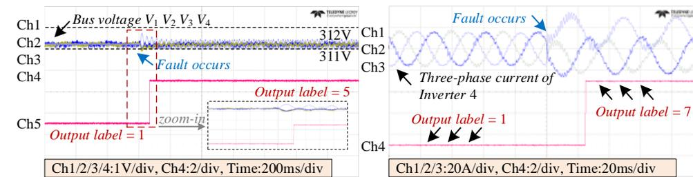
Real-time experimental results when inverter 4 is under  $T_6$  open-circuit fault (a) faulty inverter localization (b) switch fault classification.
